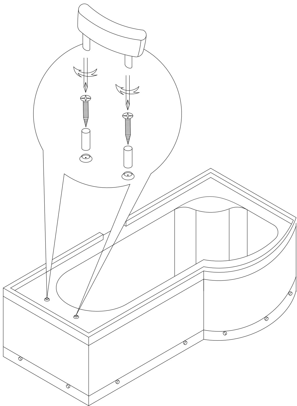
Fix the backboard on the tub with screw ST4\*12.
