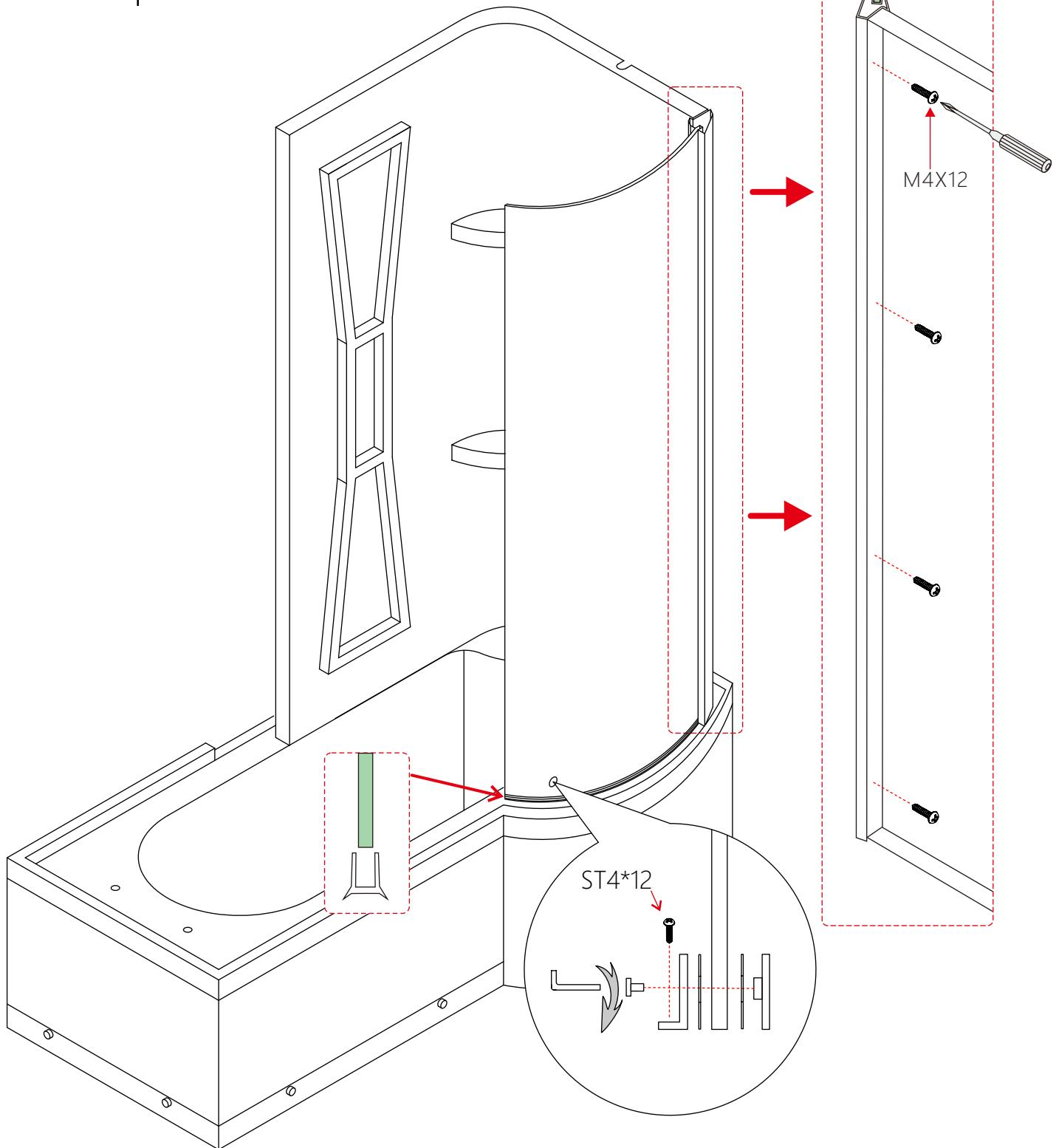
Fix the moveable glass door with screw ST4\*12 on the backboard. Then install alu minium profl to the wall.
