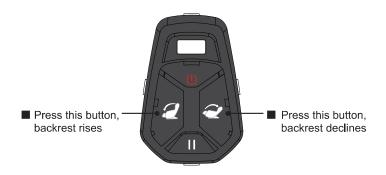
Raise and decline are the continuous movement of the chair backrest and the legrest (Stop tilting means both the backrest and the legrest)
